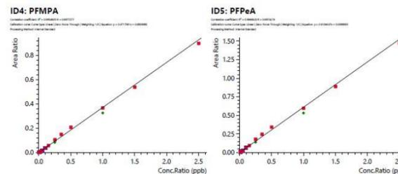
Figure 3. Aggregate calibration curves for PFMPA, and PFPeA
