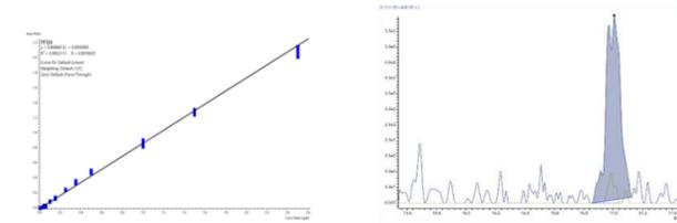
Figure 4. Aggregate calibration curve for PFDA and example MRL 0.1 ng/L chromatogram
